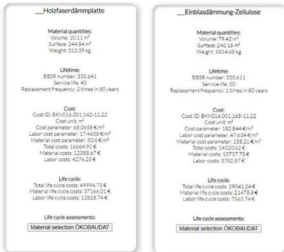
Figure 7. Example for material evaluation and material selection (left: Insulation Board, right: Cellulose Insulation)
